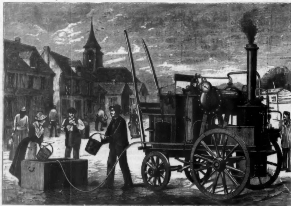
Fig. 1.—APPARATUS FOR STERILIZING WATER BY HEAT.
